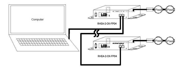
D. Online + Offline Control mode: Connect Offline main controller with computer (under this condition, computer and offline main controller do not work at the same time. Whether computer work or offline main controller work)
