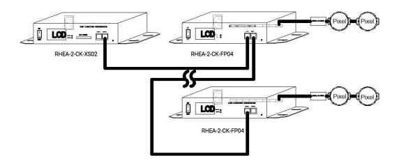
C. Online Control mode: Offline control mode can load at most 150,000 pixels, each distributor controller has 8 ports, each port can load at most 170pixels.
