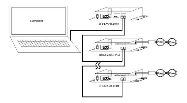
E. Large-scale project switch control: switch cascade connection can load millions of pixels, the proposed switch model is TP-LINK TL-SL2428.
