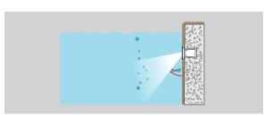
Water must be allowed to go inside and outside sleeve freely without leaking to the other side.
